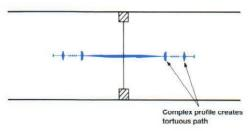
The Supercast range incorporates both of these principles. The products offer a fully continuous 4 bulbed design maintaining both the valve and tortuous path principles. These principles are maintained in the transition from Rearguard profiles in floors to centrally placed profiles in walls.
